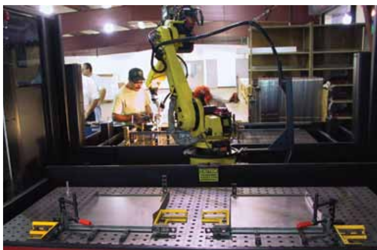
Figure 5. Modular fixturing makes it feasible for robots to weld simple parts with low lot sizes by having the setup technician and welding operator trade places setting and welding throughout the day.
