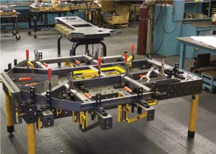
Figure 3. A modular fixture serves as the first in-process quality check for all of the loose pieces.
