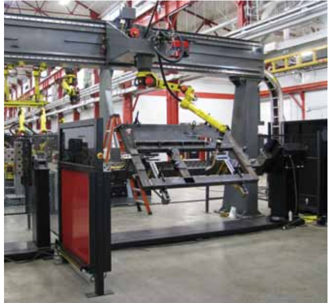
Figure 6. When gantry robots are used to weld larger parts, the modular fixturing consists of a square spacer block with a full pattern of system bores on three sides and the two ends. Mounted between a headstock and a tailstock, the robot is able to access all sides of the part.
