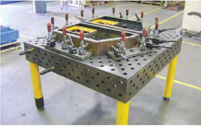
Modular fixture built from the CAD model.
