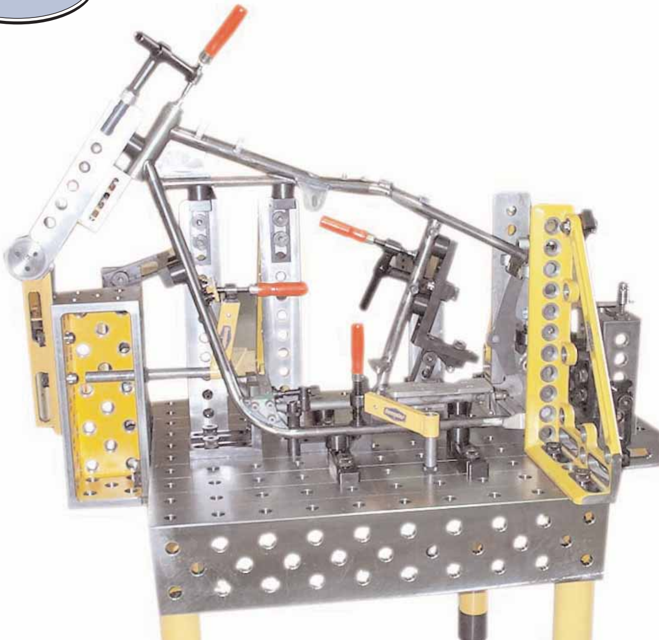
Motorcycle frame fixtured on a 1000 x 1000mm (40" x 40") D28 table
