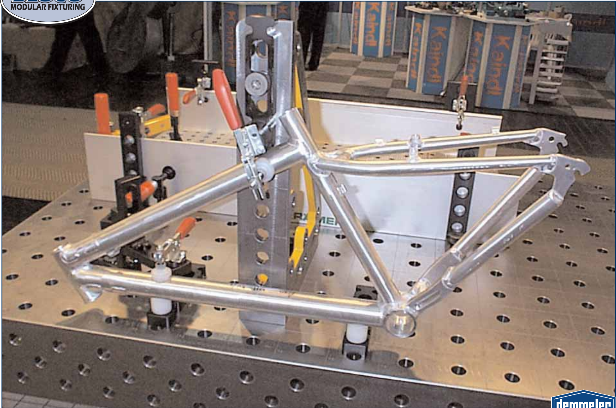
Bike frame held with nylon v-blocks and clamping pads to keep from damaging finish
