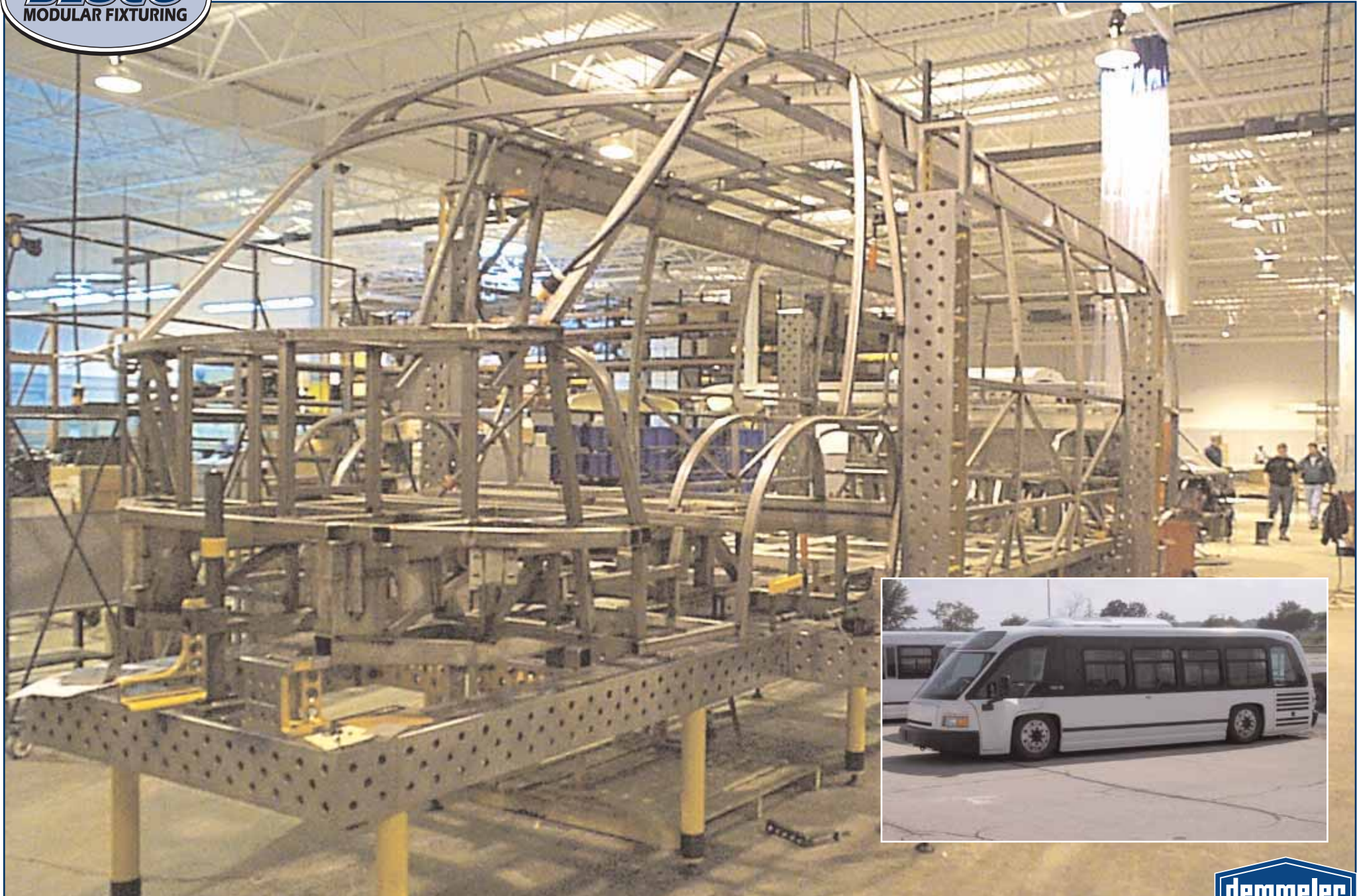
Final assembly fixture for 30' stainless steel bus frame.
