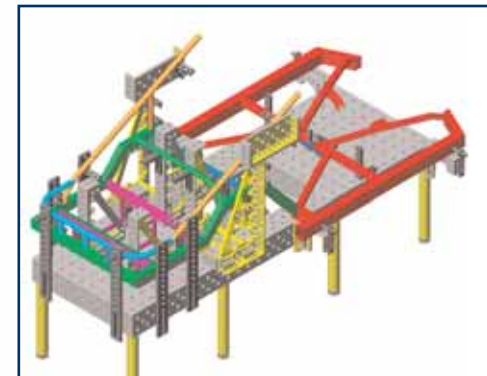
NASCAR chassis built in sub-assemblies (front clip, roll cage, rear clip)
