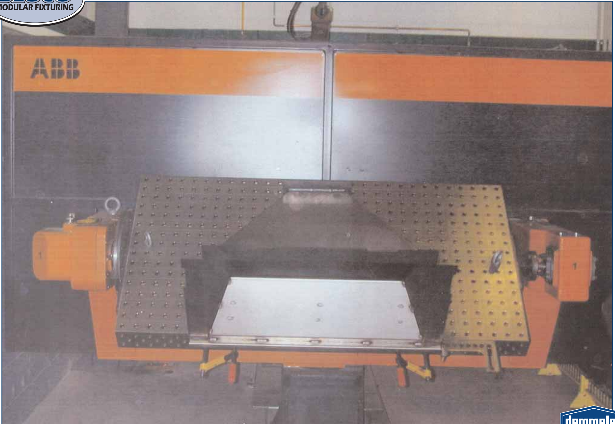
A standard D16 1000 x 2000 mm (40" x 80") table with its legs removed is used in this rollover fixture
