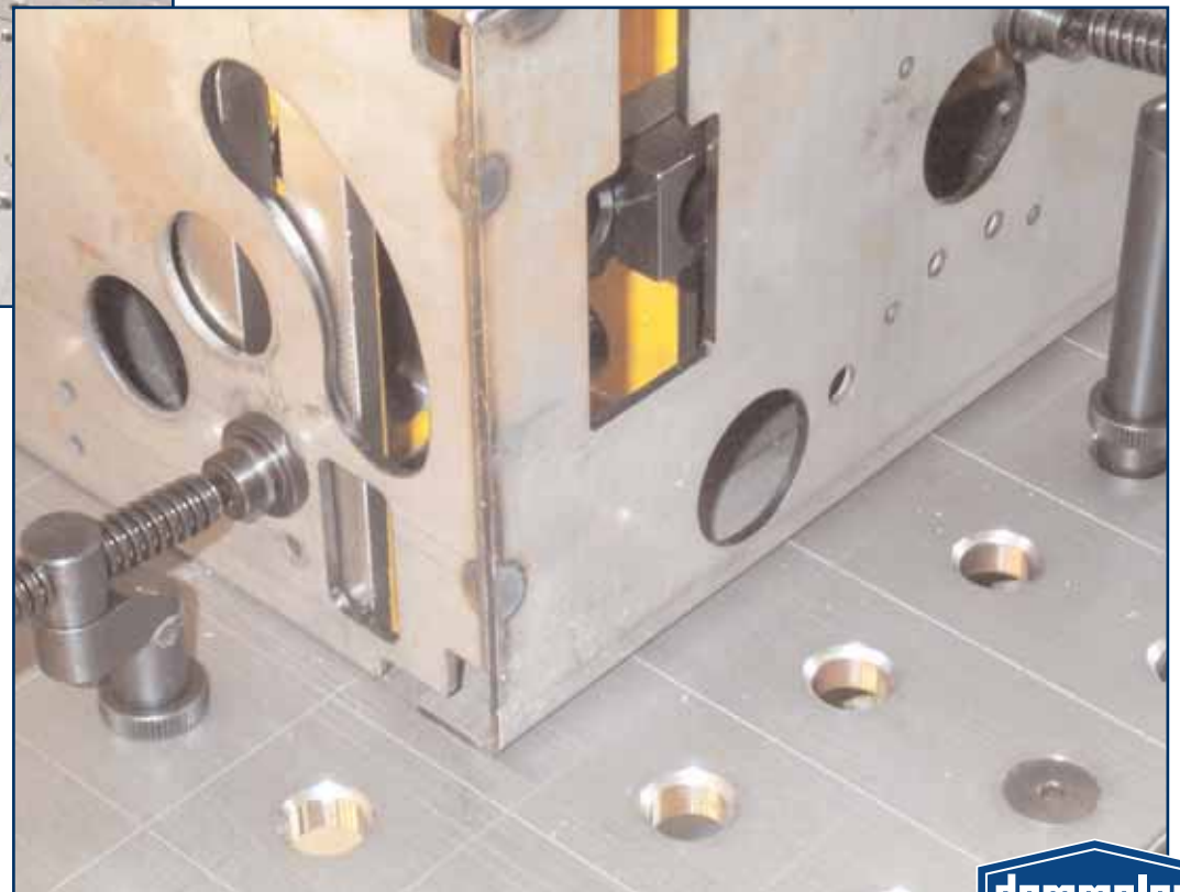
Welding fixture set up for Trumpf laser
