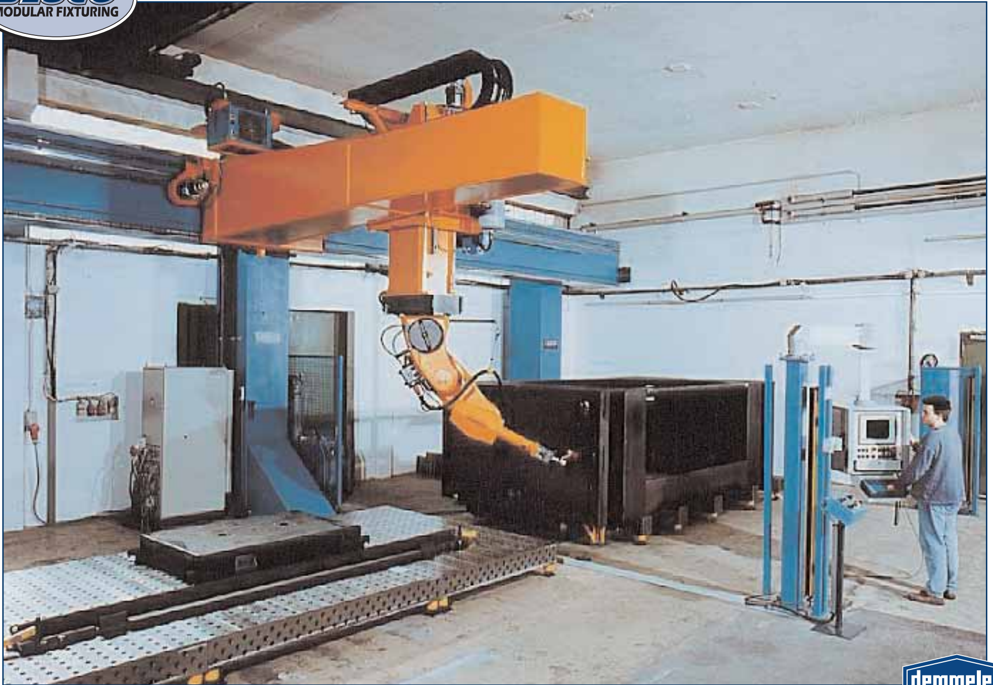
Multiple tables are joined together in front of a traveling gantry robot
