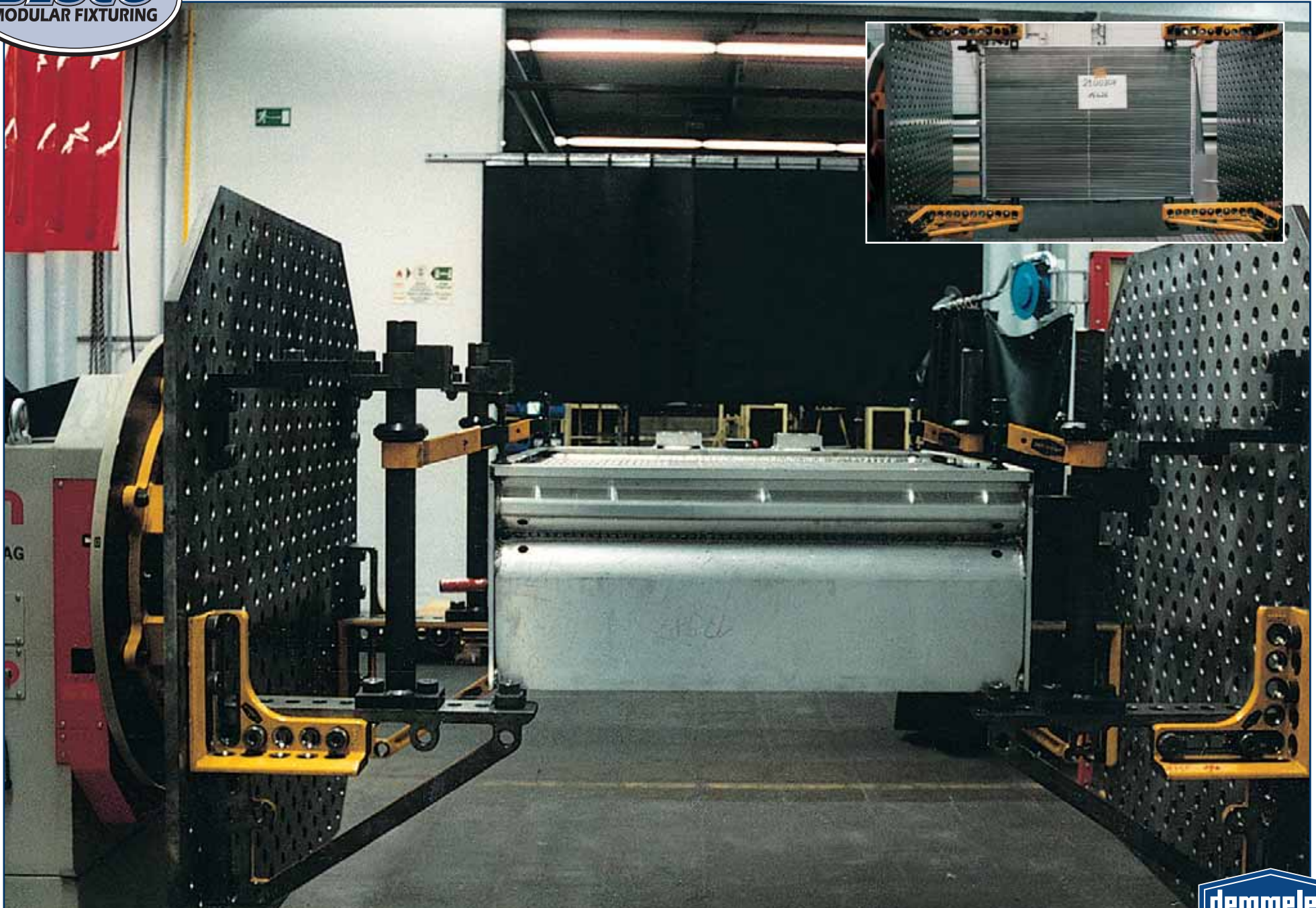
Twin plate (left and right) are attached to rotary tables and used to hold radiators
