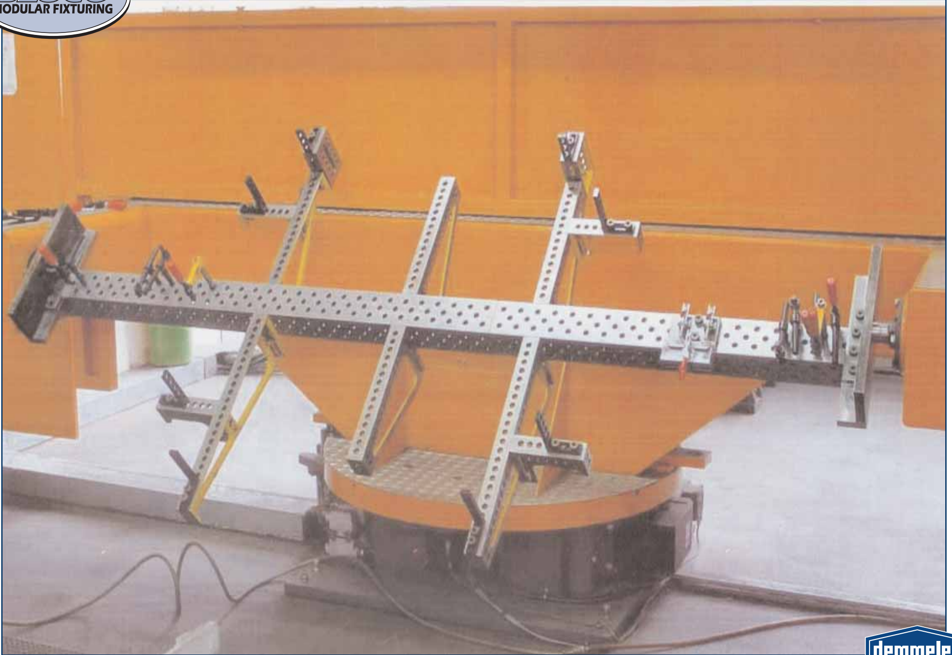
A single U-form spacer block acts as a “spine” to hold outriggers (angles) where needed
