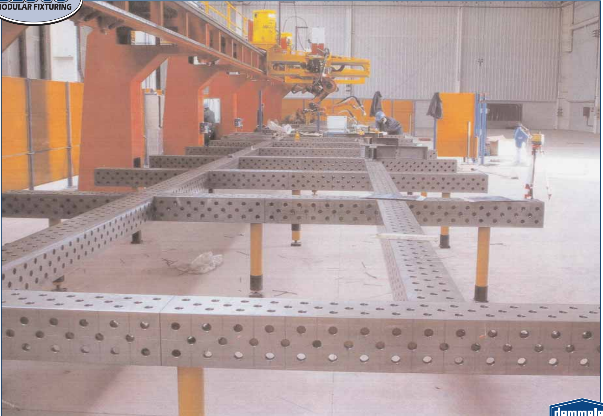
U-Form spacer blocks provide plenty of access for overhead traveling robotic welding
