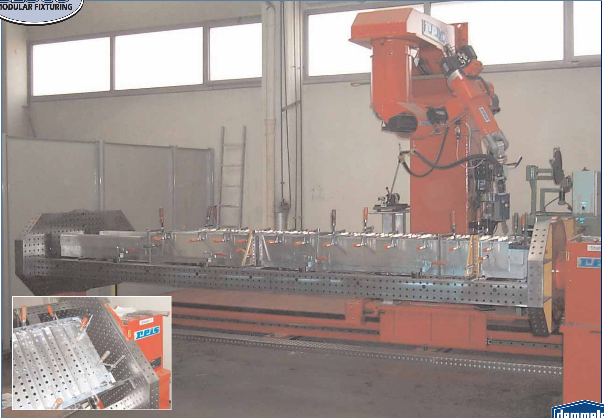
Head and tail stock with modular tables attached supports long u-form block for rollover fixture
