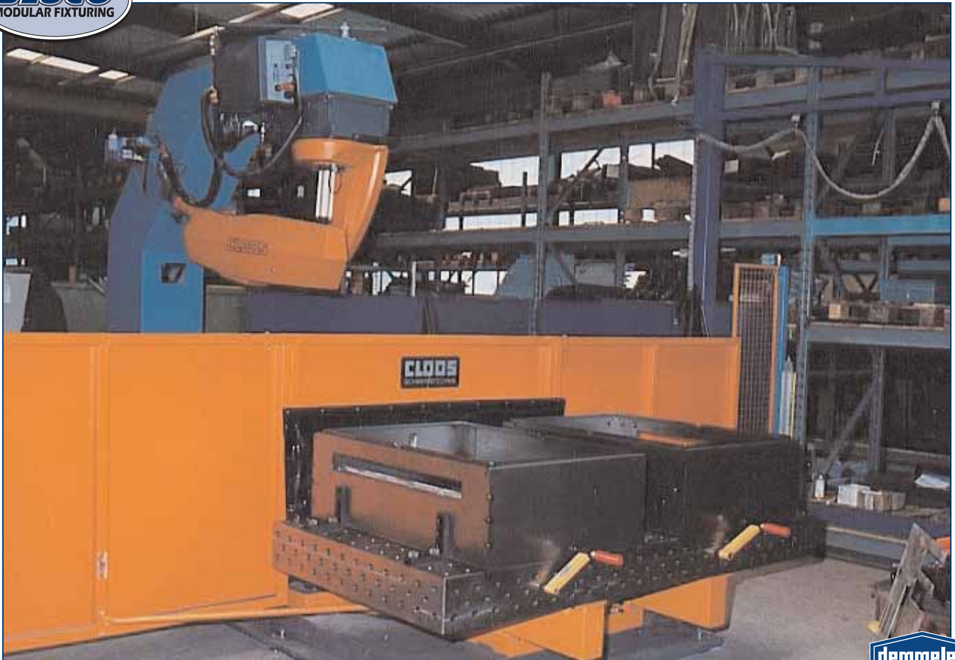
Two 1000 x 2000mm (40" x 80") tables without legs are used as the base for this rotary pallet changer
