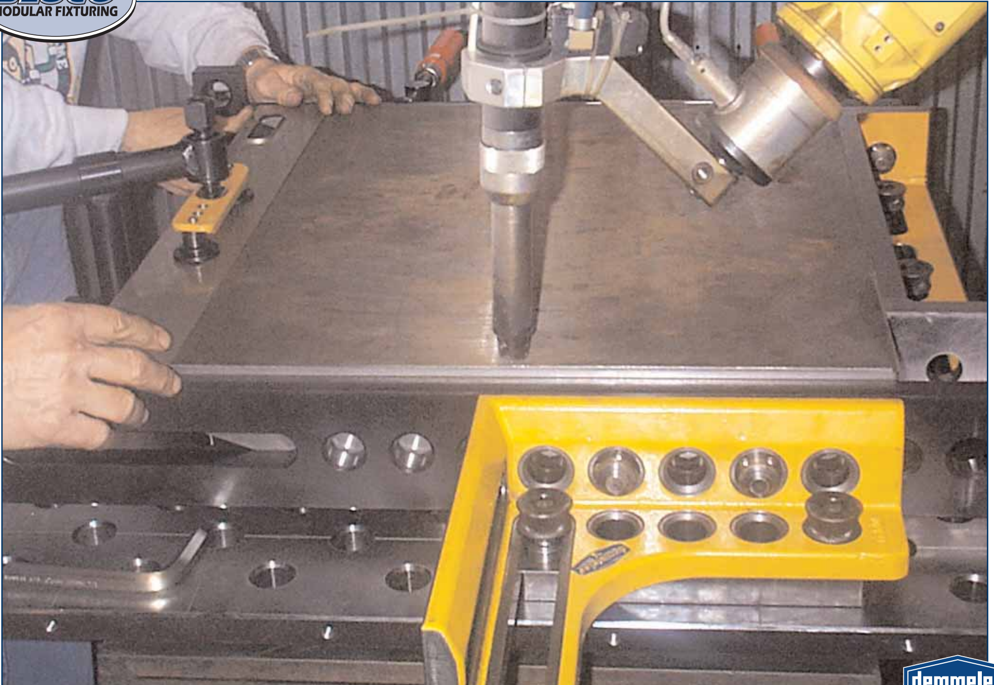
Hamburger grill is fixtured upside down with all four edges square for robotic welding
