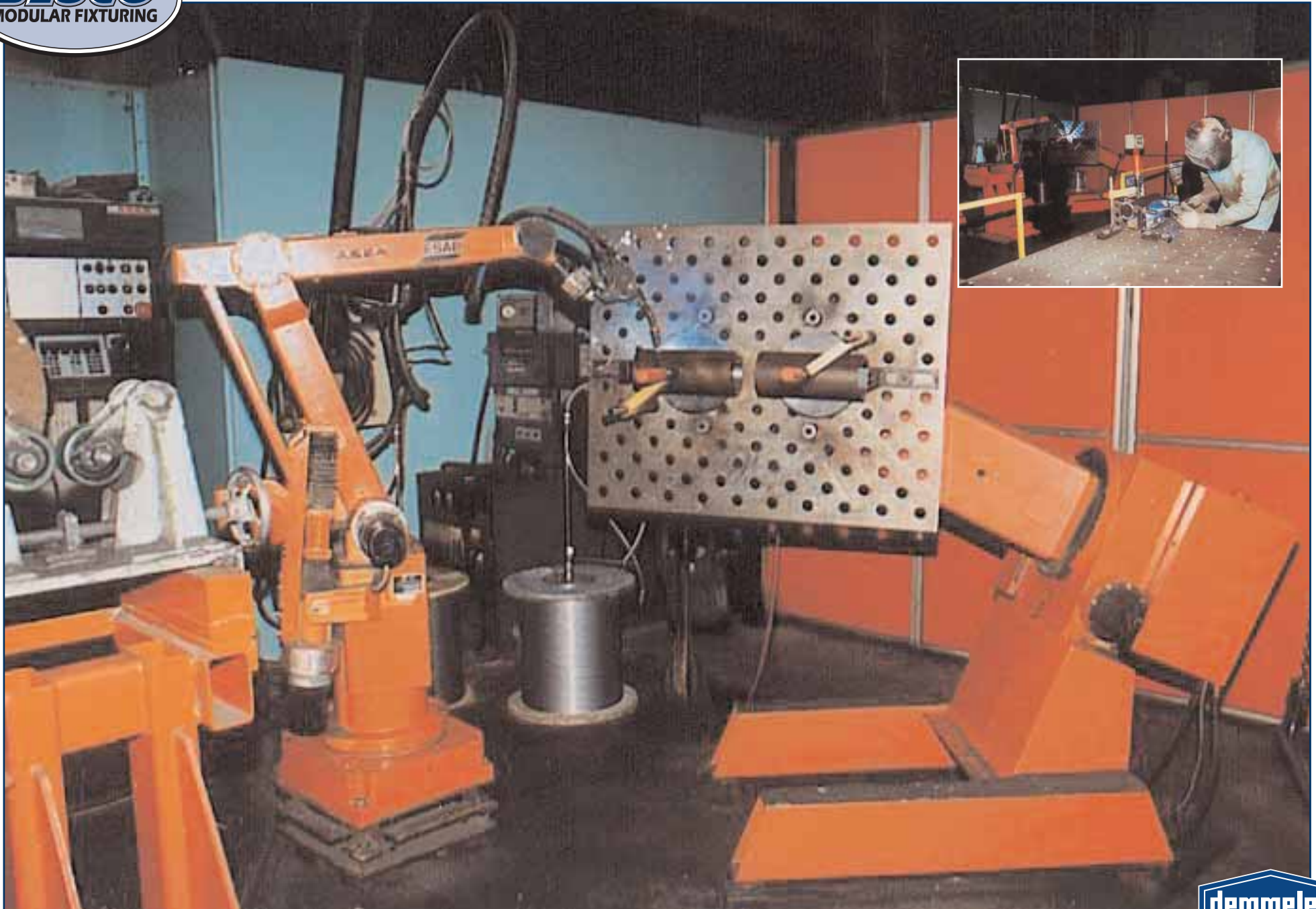
Welder pre-tacks part in a modular fixture before loading into robot cell
