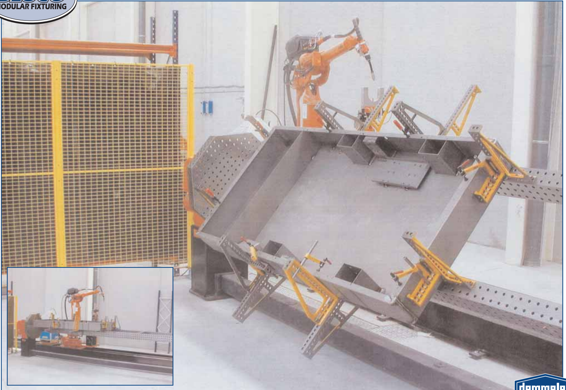
A pair of U-form spacer blocks span the entire length to allow for access on both sides of the sheetmetal cabinet
