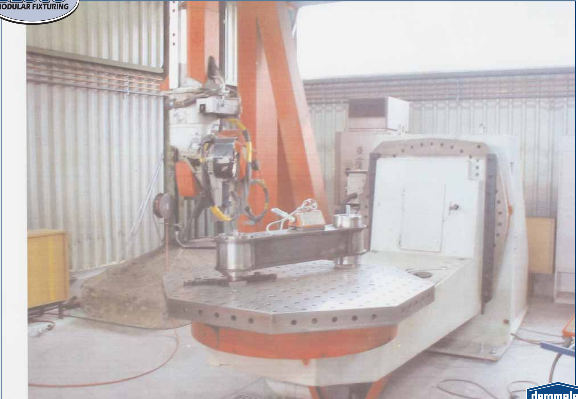
Modular table sits atop a tilt and rotate positioner for short run robotic parts
