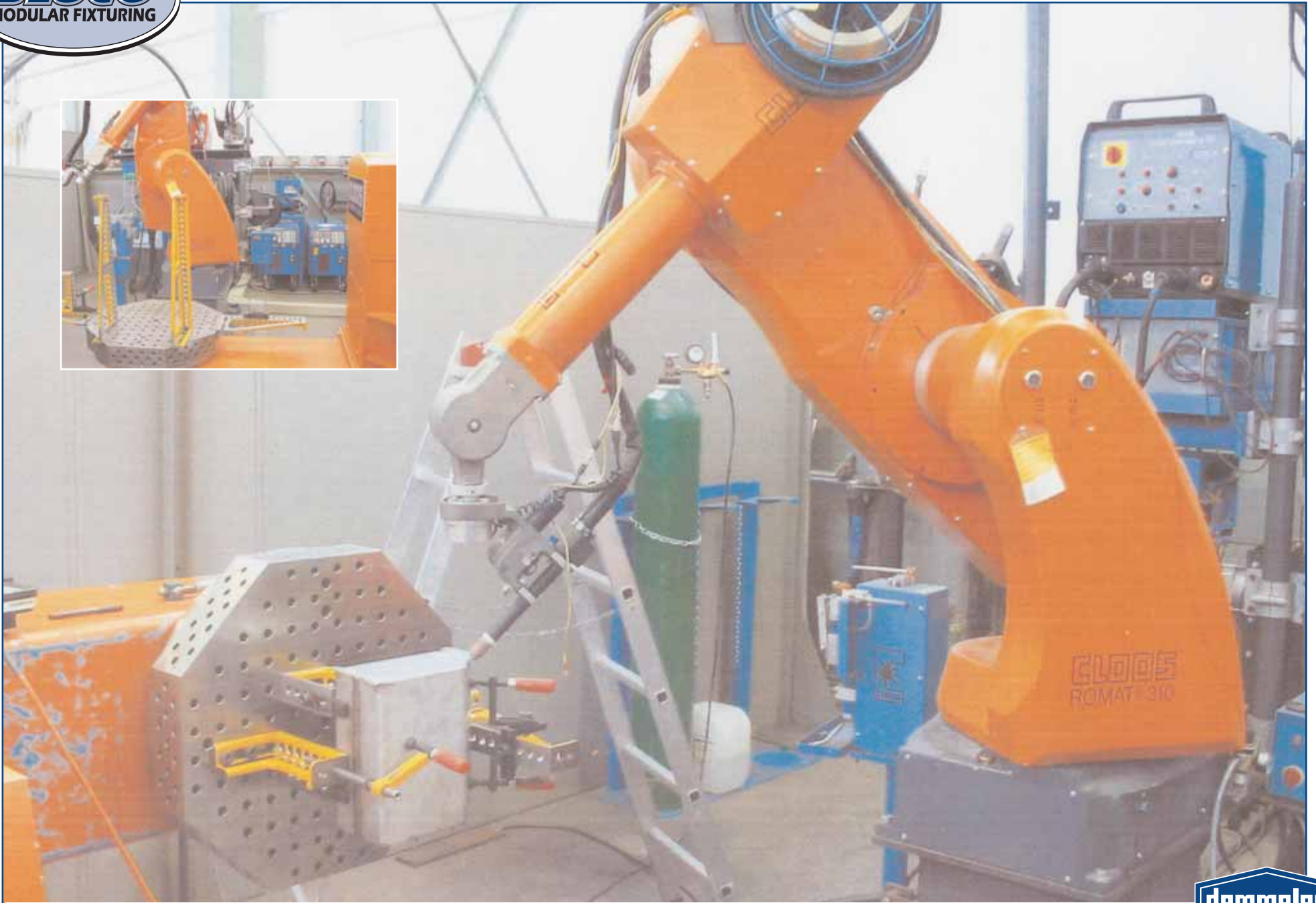
Small, octagonal table in front of robot rotates for full robot access
