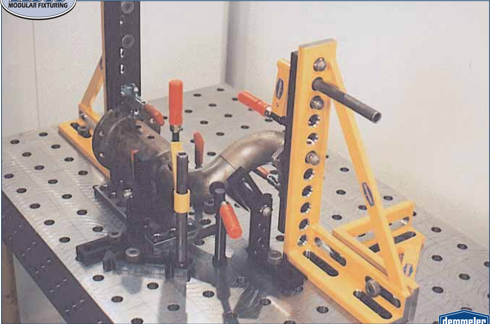
Small exhaust assembly has three flanges all aligned (two on the ends, one on the bottom)
