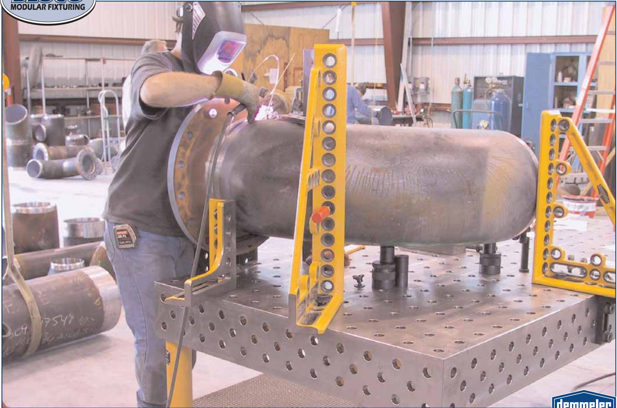
Locating bars square up the large flange while large angles align the pipe
