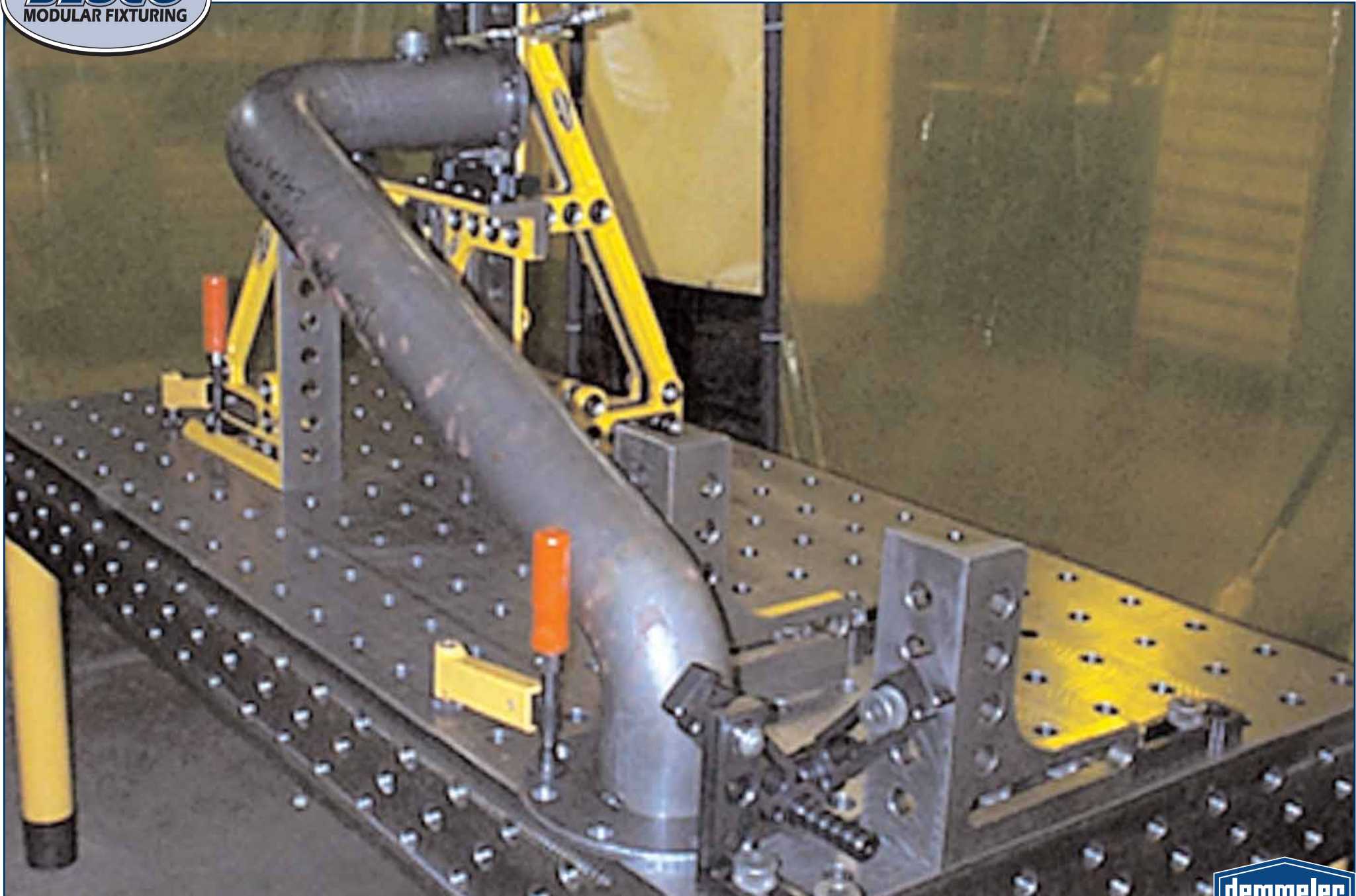
Exhaust header has two flanges in separate planes accurately located
